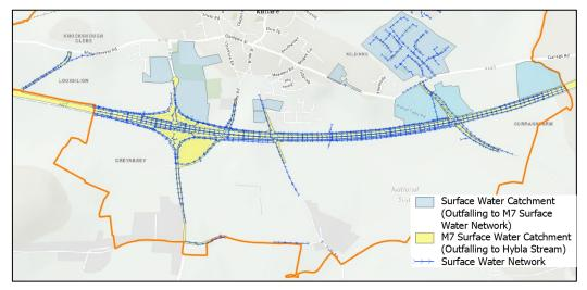
Figure 6-3 M7 Drainage Network and Connected Areas
